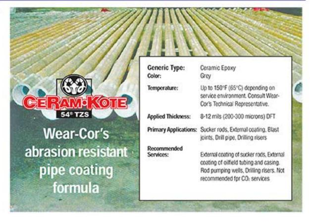
CeRam-Kote 54® TZS is a thin-film, spray applied ceramic epoxy coating engineered primarily to provide external abrasion resistance and corrosion protection. CeRam-Kote 54® TZS is a highly modified epoxy resin system that has been heavily loaded with a unique package of ceramic particles enhancing its ability to perform well in a variety of abrasive environments.
